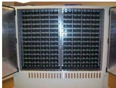
The above picture shows Flexstar's green 416B fully populated with all 416 drives. The new Green 416B is five times faster than its predecessor - enabling Flexstar customers to increase production capabilities by testing more drives in less time.
